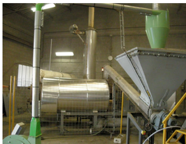
Pyro-6F machine producing biochar in a continuous way
