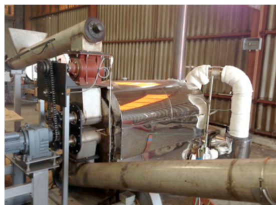
Carbonizer Pyrochar-1 producing biochar
